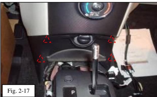
(p) Remove front console box cover by disengaging 4 clips and pulling toward the shifter along the 2 guides. (Fig. 2-17)
