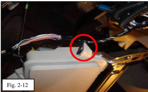
(i) If necessary, disengage wire harness clip from airbag panel to give more slack. (Fig 2-12)
